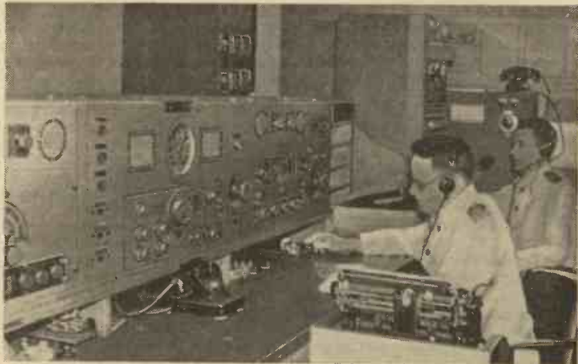
THE WIRELESS OFFICE on board S.S. America, now the United States transport West Point . The nine-foot console incorporates the controls of the three main R.C.A. radio-telegraph transmitters, whilst that at which the farther operator is sitting is the radio-telephone control panel. The three CW transmitters each have a power of 1 kW. and work on the short-, medium- and long-wave bands. The main console also has an aerial switching panel providing the selection of any of the five receiving doublets for either of the two high-frequency receivers. The ship's complete radio equipment includes eight transmitters, nine receivers, a direction finder, an automatic distress alarm and thirteen aerials.
